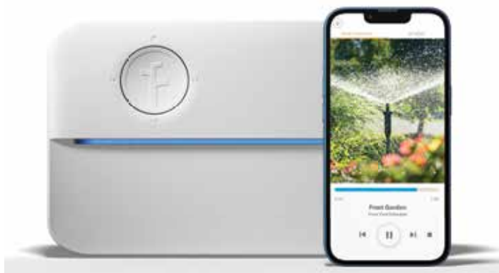
Figure 1. The Rachio is a WBIC that leverages internet access from existing Wi-Fi networks to obtain ET and rainfall information for scheduling irrigation. Image downloaded from https://rachio.com/newsroom/
